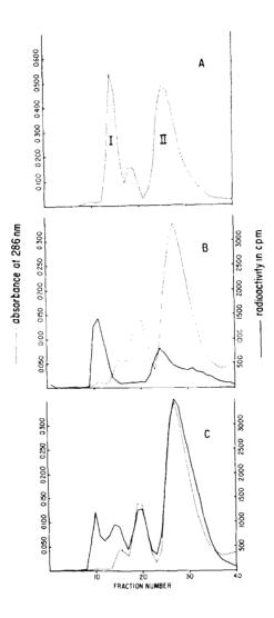
Fig. 2 A. Separation of cis(I) and trans(II) phytoene on a 1% deactivated alumina. A linear gradient of Skellysolve B to 9% diethyl ether in Skellysolve B was used for column elution. Five-milliliter fractions were collected.
